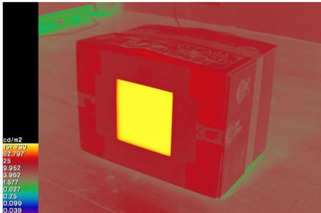
Figure 2: False colour image of the light source
