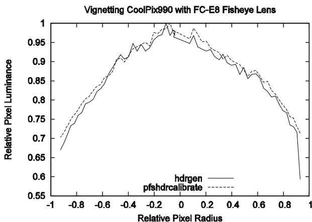
Figure 7: Pixel intensity vs distance from image centre
