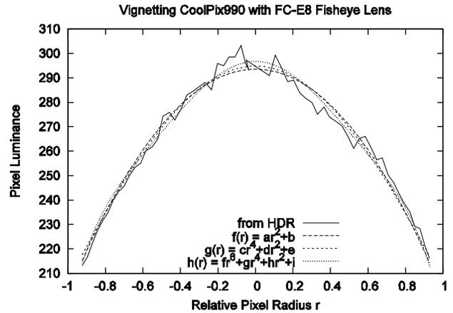
Figure 8: Curve-fit of the vignetting drop-off (*pfstools*)
