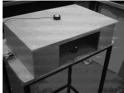
Fig 7: Model B4 turned around with a full height window and complies with the limiting depth criteria. For measured results see table 4
