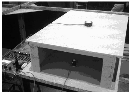
Fig 5: Model A4 with full height window. This model does not comply with the limiting depth criteria. For measured results see table 2.
