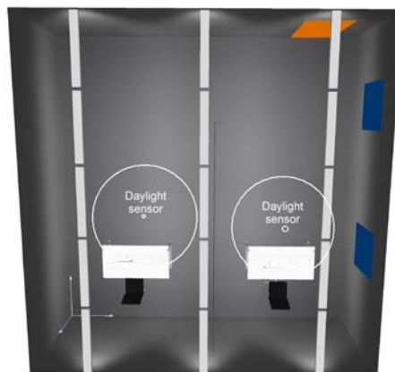
Placement of sensors
