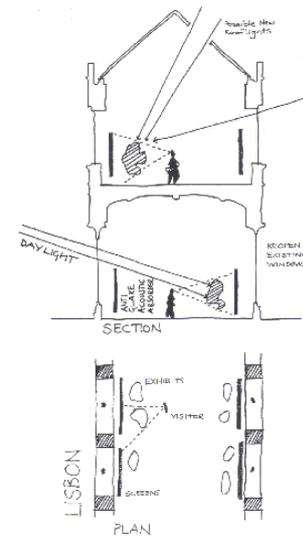
**Illustration 5:** Cross-section and detail of the plan after the refitting.
